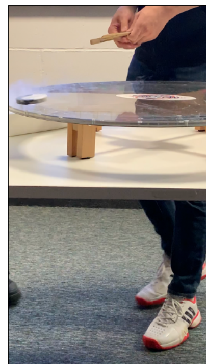
A superconducting puck, cooled by liquid nitrogen, floats above a ring of magnets.
